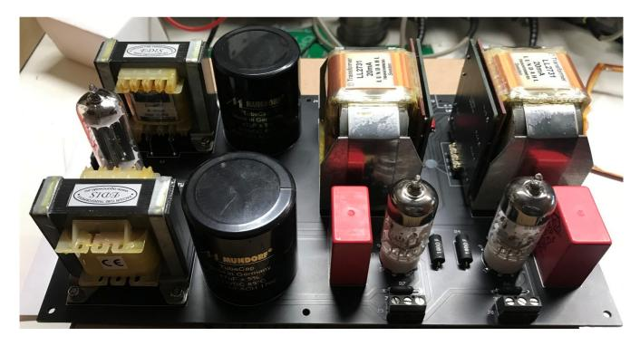
Vacuum tube line buffer suitable to be used as impedance adapter for voltage output DAC..
