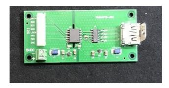
The board receives I2S signals over HDMI cable. The purpose of this board is to keep the I2S source far from the DAC. The I2S input is LVDS, the I2S output is single-ended CMOS.
