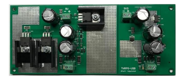
Low noise voltage shunt regulator designed to provide power supply to TWSAFB-XMOS I2S/DSD over USB interface.
